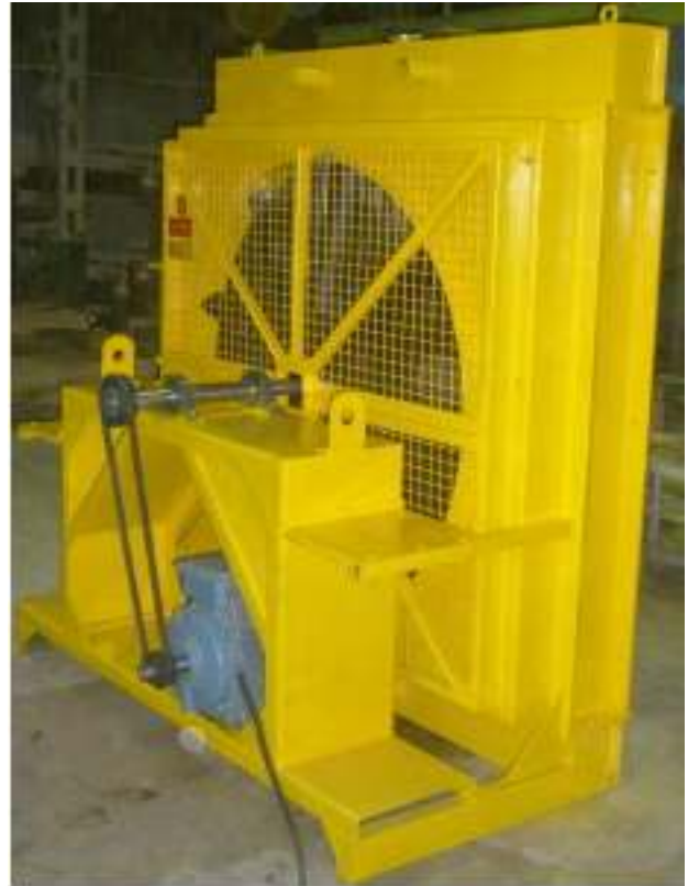
Radiators with Fan Mounted on Pulley & shaft
