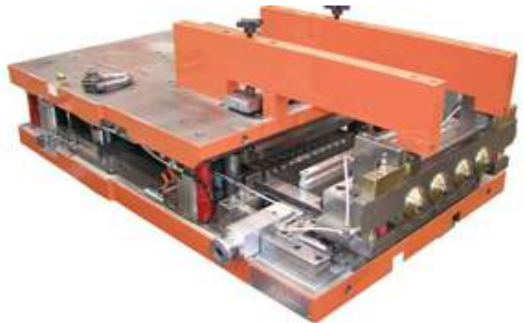
Fins are punched on Burr Oak , USA die . This is the best die available in today's world.
